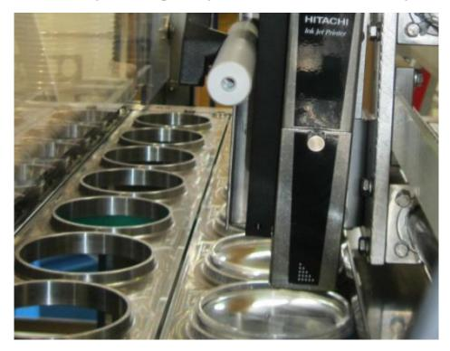
IMS-Partners and Van Alstine, with deep experience fitting Hitachi printers into food manufacturing, worked together with Hitachi to establish the solution's viability for Kraft. The Hitachi RX SD160W ran 3 hours 20 minutes in tests without any issues or faults. The printhead remained clean and the print quality was outstanding.
