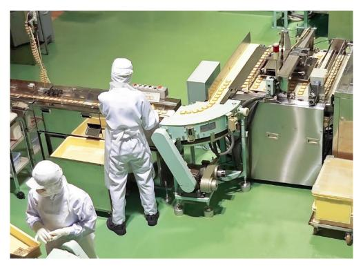
Marking and Coding is a necessary step in virtually all bakery and confectionery production processes. While just one part of the overall process, unless carefully considered this step can negatively influence your ability to meet production targets in significant ways.
